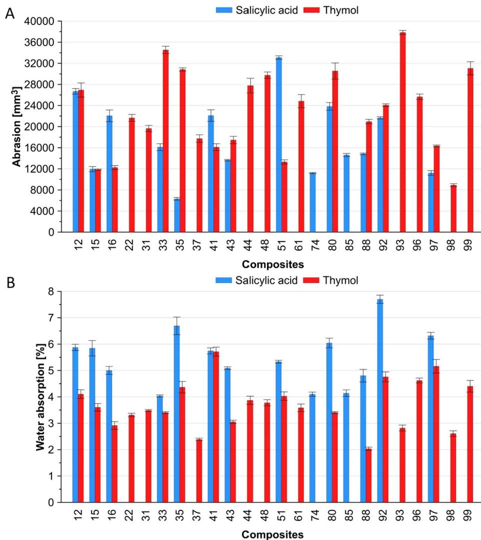
The composites also showed variations in abrasion resistance and soakability (Fig. 6A and B). For example, the 35SA composite had a low abrasion resistance of about 6300 mm<sup>3</sup> but a high soaking capacity of 6.7%. In contrast, the abrasion resistance of the 93 T thymol-added composite was almost 38,000 mm<sup>3</sup> and the soakability was only 2.8%.
