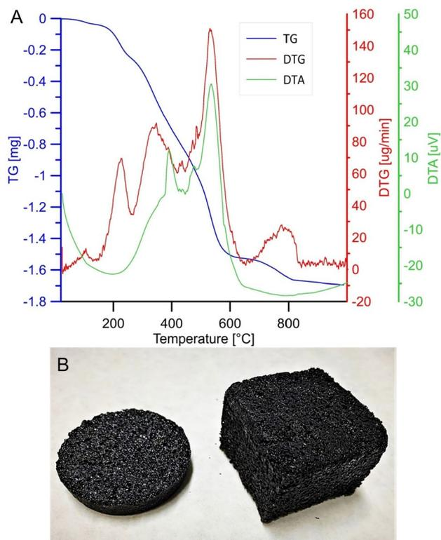
**Fig. 2** Composite No. 98SA: **A** thermogravimetric/differential thermal analysis; **B** photograph
